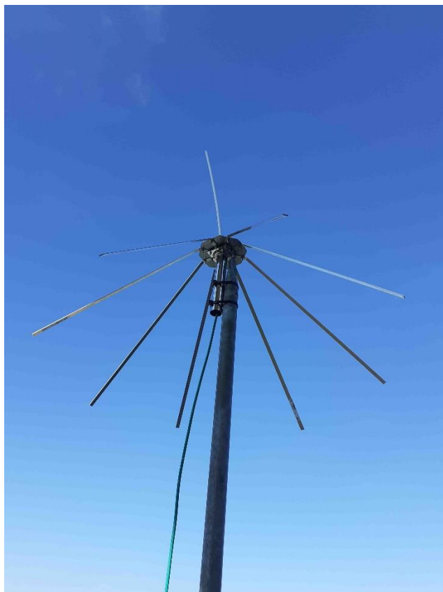
Figure 17 – Testing of the self-built ground plane antenna.
